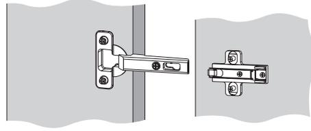
Turn screws as shown to adjust door position
