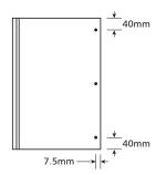
Now fix the Door Post **9** to the front inside edge of the side panel, using 3 x screw **6**.
