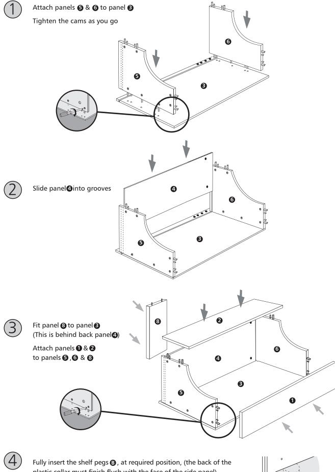
plastic collar must finish flush with the face of the side panel).
