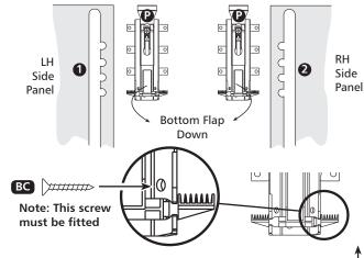
Turn screwdriver ② anticlockwise to increase height
