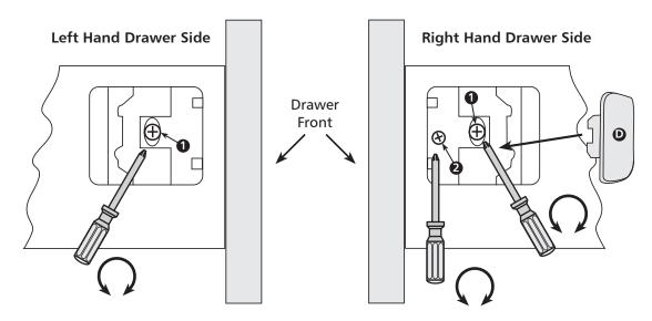
For **Vertical** adjustment, loosen screws **1** adjust Drawer front to desired position, re-tighten screws **1**.
